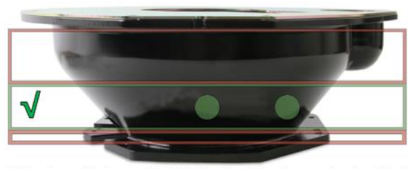
Two 1.75 inch round holes may be drilled in the defined area under the following conditions: The outside of the holes must be separated by a minimum of 2 inches, The outside of the holes are not drilled within one inch of any other opening. The outside of the holes must remain inside the defined area.
