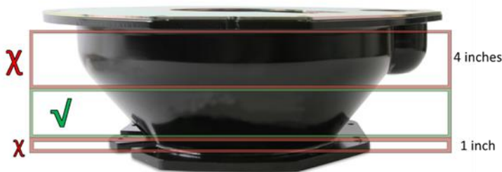
Modifications may be made in the area a minimum of 4 inches from the back side of the engine flange and a minimum of 1 inch from the front side of the transmission flange.
